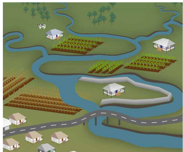
Figure 72. Poorly planned artificial levees can increase likelihood of channel avulsion
